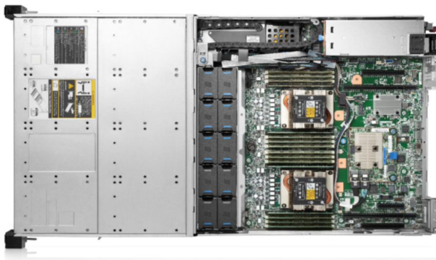
FIGURE 2. HPE Apollo 4200 Gen10 server with dual processors and fully populated RAM
